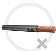
Damaged conductor insulation
