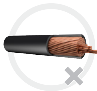
Pulled out conductor
